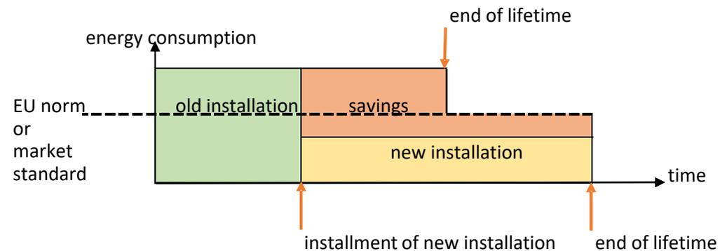
Figure 1: Schematic visualisation for determining energy savings in the case of early replacement
