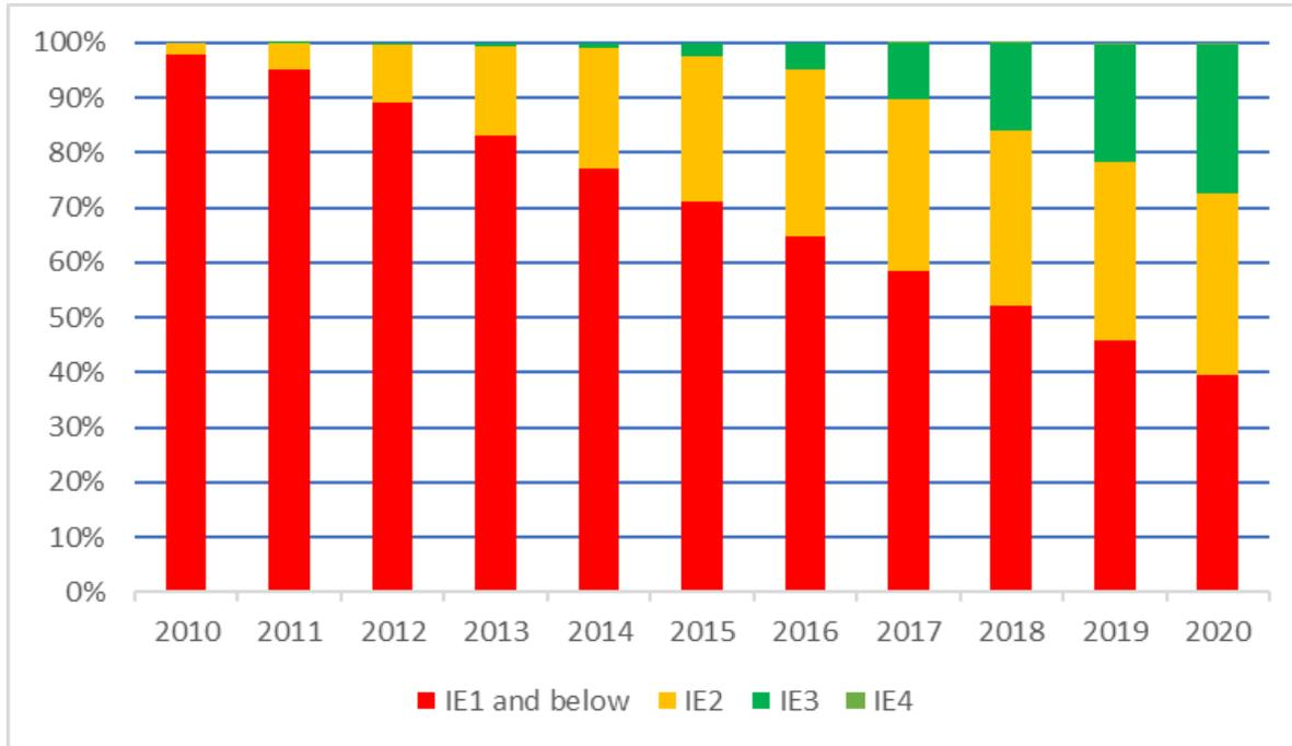
Even when taking the values of 12, 15 and 20 years for the average lifetime, depending on motor power range, it can be seen that, despite the Ecodesign Regulation in place, over 70% of the motors installed in the EU-27 were still IE2 efficiency class or below in 2020
