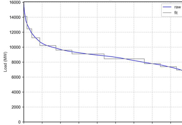
Figure 2: Load duration curve and the associated loadblock functional approximation.
