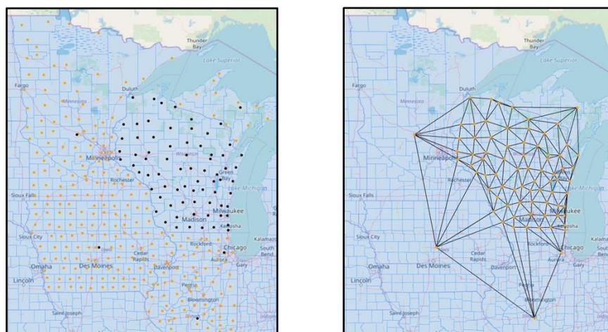
Figure 1: (LEFT) A map of the disaggregated node system in the model (orange markers) alongside the aggregated boundary node system (black markers). (RIGHT) A map of the synthetic transmission network that was created from the automated triangulation methods.
