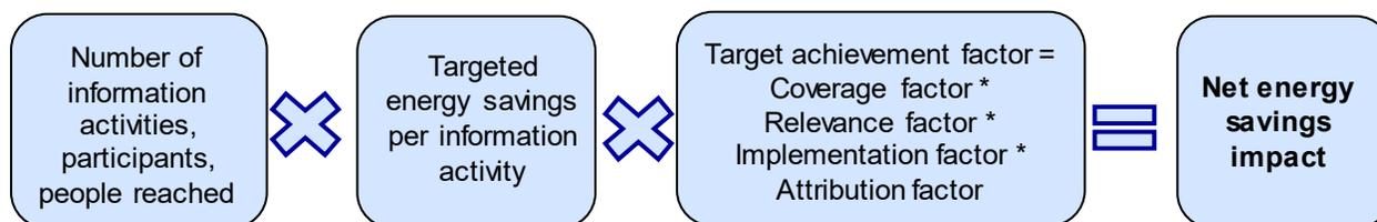
Figure 3. Energy savings impact chain of multi-stage evaluation model by VZ NRW
