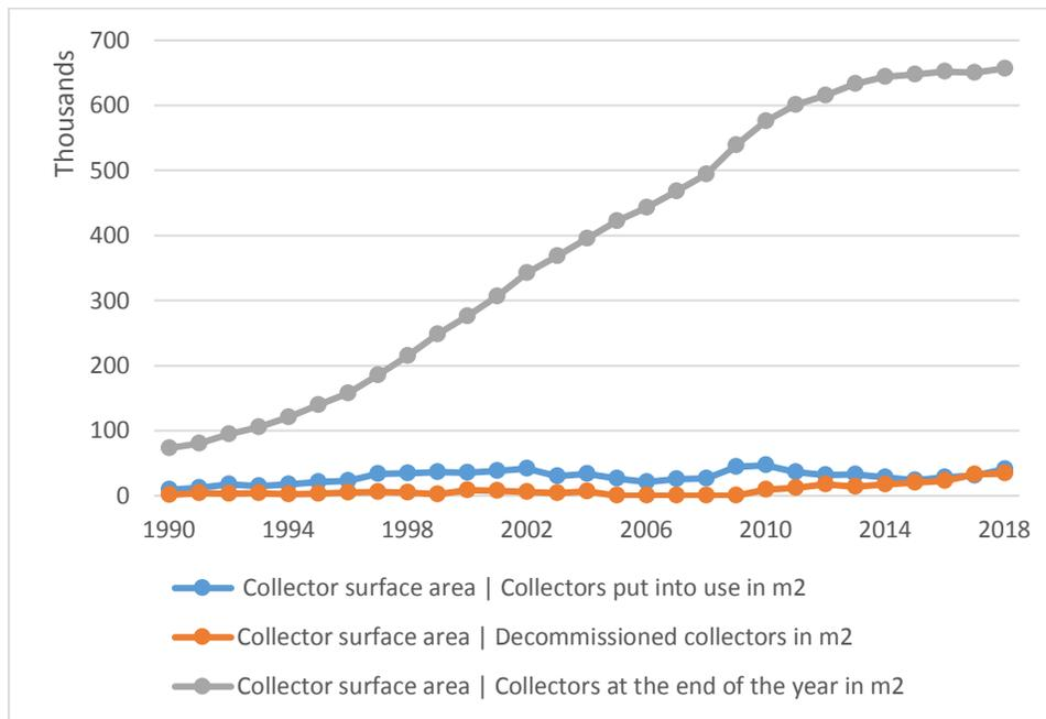
Figure 3 Total surface area (m<sup>2</sup>) of solar collectors producing heat in both residential and non-residential buildings (CBS, 2020b)
