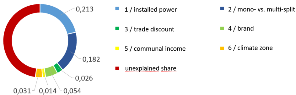
Figure 1: Change in the coefficient of determination (R 2 adj = 0.52) according to the variable selected (stepwise procedure) for the air/air HP "technical sample" (price in €/m 2 excluding VAT). The segments show the coefficient of determination increase by the cumulative addition of a new variable.
