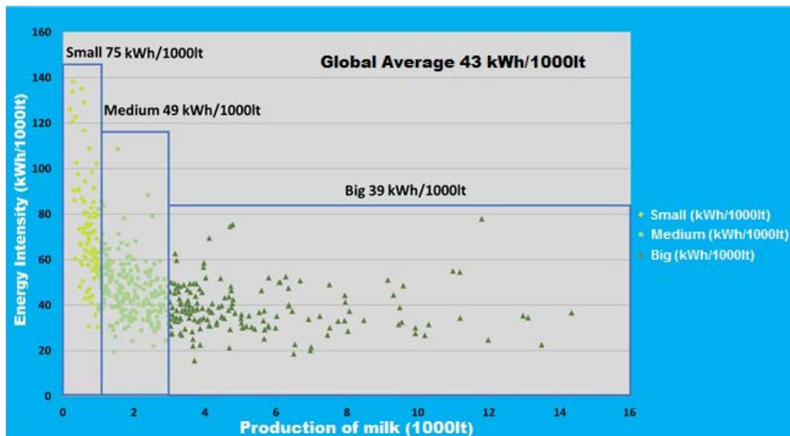
Figure 3: Energy intensity vs. daily milk production.
