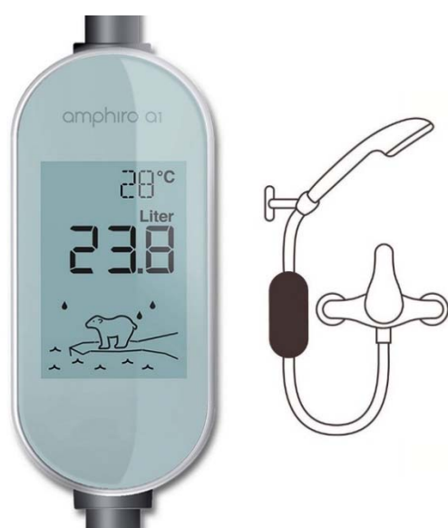
Figure 1. The smart shower meter displays feedback on energy and water use in real time in the shower, toggling different display elements (e.g., temperature and energy efficiency class). The image on the left shows a snapshot of the feedback displayed; the drawing on the right illustrates the position of the device in the shower.
