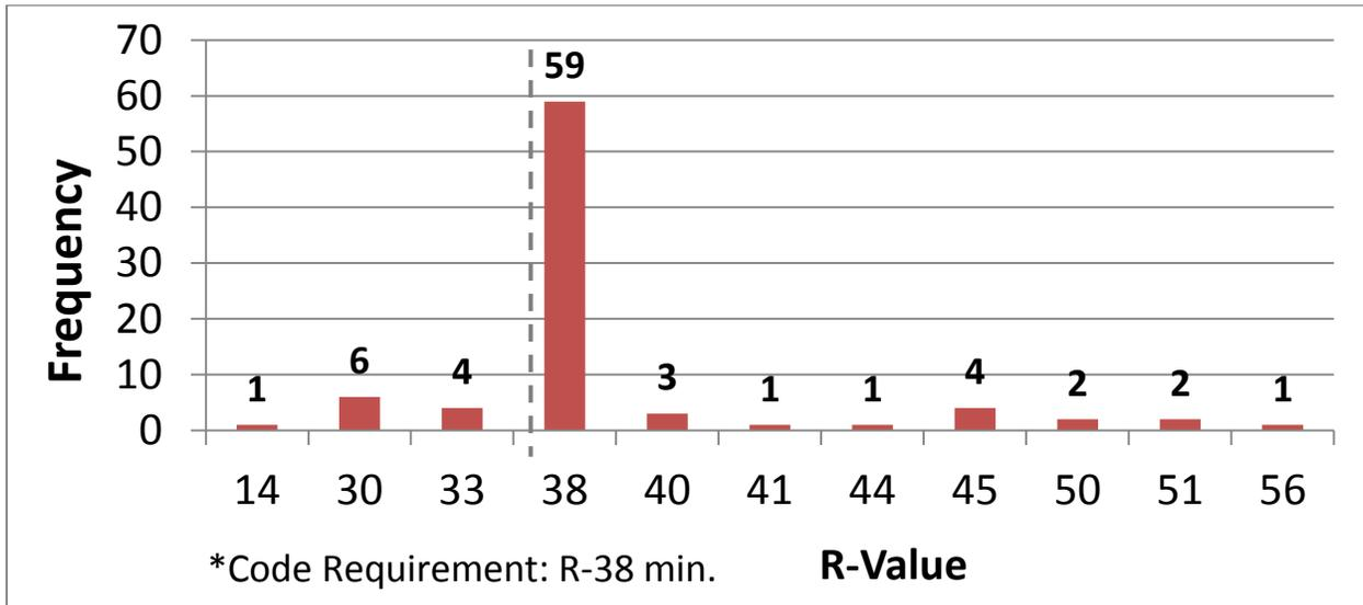
Figure 8. Ceiling Insulation R-Value
