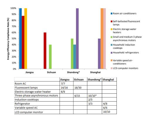
Figure 1. 2009 Energy Efficiency Check-Testing Compliance Results by Product and Region Note: Shandong's motor compliance rate is shown in the graph as nominal efficiency only, but was reported as 100% (and shown in table) to account for tolerance of additional losses between nominal and minimum guaranteed efficiency. Data Source: Jiangsu QTSB 2010, Sichuan IQITR 2010, Shandong IQITR 2011, Shanghai IQITR 2011
